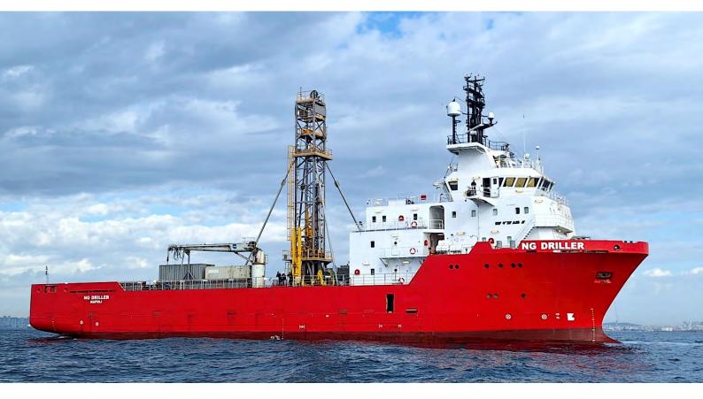
The NG Driller is a DP2 geotechnical survey vessel with 70tons drilling tower on the moonpool permanently installed to perform the following activities:
